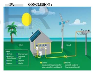
The benefit of using this kind of system is that it can cut our electricity bills as we are feeding back the part of the energy. It is done by synchronizing our power to the grid connected.
